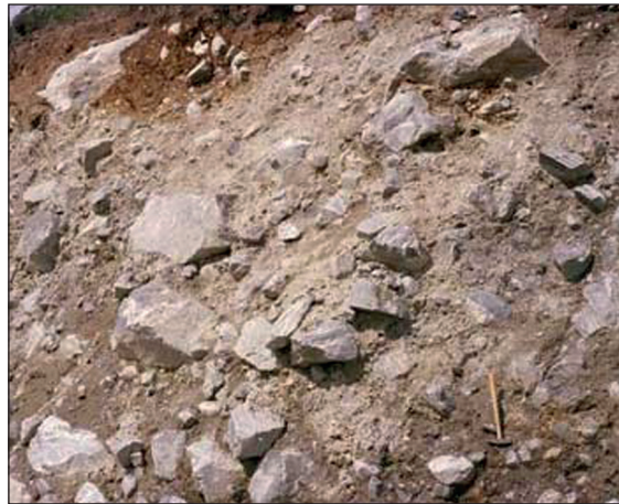
Quaternary till with angular grains. Grains vary in size from less than 0.05 mm up to 50 cm.
